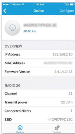
**Configure** To manage the device, go to the *Configure* section in the next column.
